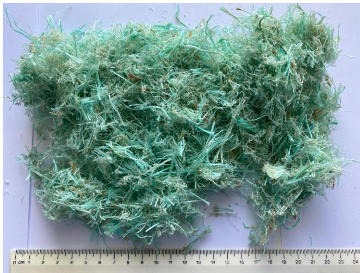
Figure 11. Shredded polypropylene fibres from rope
