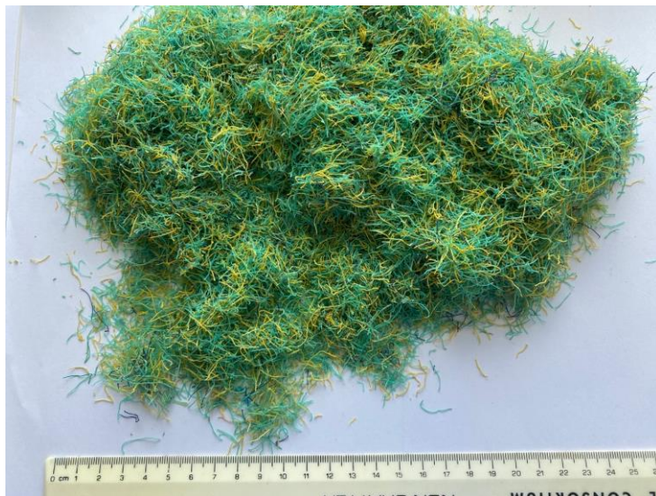
Figure 12. Shredded HDPE fibres from trawl net
